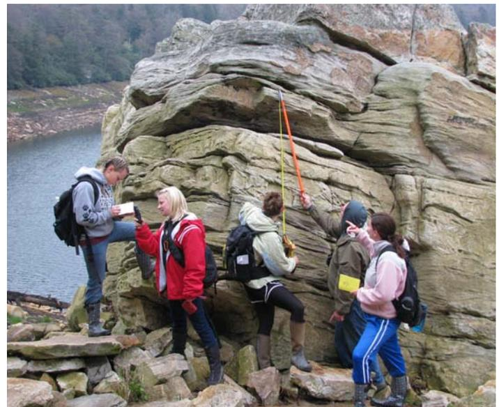
Dr. Carl Friese and a team of students enrolled in the new INSS field course measure the decrease in the water level height of Mountain Lake in Virginia with meter tapes and GPS. The water level of the lake used to be just below the top of the boulder they are measuring.
