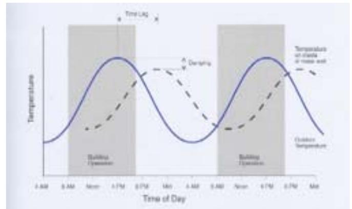
Figure 1. Damping and lag effect of thermal mass [1].
