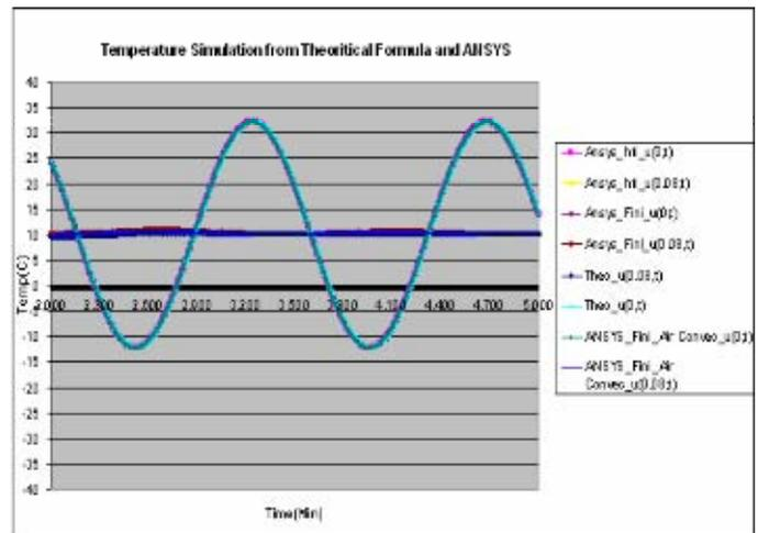
Figure 7. Comparison of analytical and finite element results for an infinite and finite wall at 0.08 meters.
