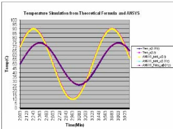
Figure 6. Comparison of analytical and finite element results for an infinite and finite wall at 0.01 meters.
