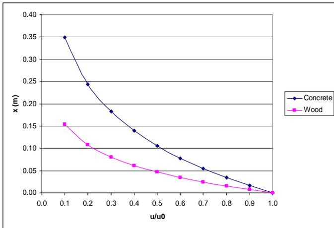
Figure 8. Amplitude dampening for wood and concrete walls
