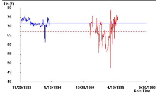
Figure 5. Inside air temperatures from December through April of the baseline and post-retrofit period
