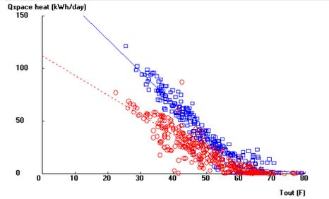
Figure 3. Pre (square) and post-retrofit (circle), daily space-heating energy consumption plotted against outside temperature for mobile home 314 in Shelton Washington and fit with four-parameter regression models.
