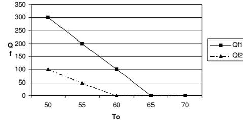
Figure 1. Expected traces of baseline (1) and post-retrofit (2) furnace heat into a building versus outdoor air temperature when  $UA$  decreases as a result of a weatherization retrofit and  $T_i$  and  $Q_i$  remain constant.
