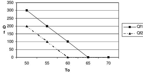
Figure 2. Traces of baseline (1) and post-retrofit (2) furnace heat into a building versus outdoor air temperature when the building UA remains unchanged, but either  $T_i$  decreases from 70 F (21.1 C) to 65 F (18.3 C) or  $Q_i$  increases from 100 to 200. The decreased energy consumption during the post-retrofit period is caused by changing  $T_i$  and  $Q_i$ .
