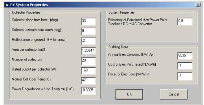
Figure 11. PV system inputs for SolarSim.
