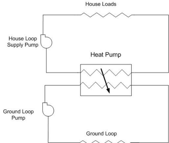
Figure 5. Geothermal heat pump schematic.
