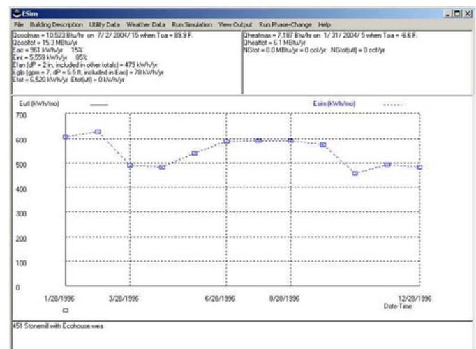
Figure 8. Simulated electricity use for the Eco-house.
