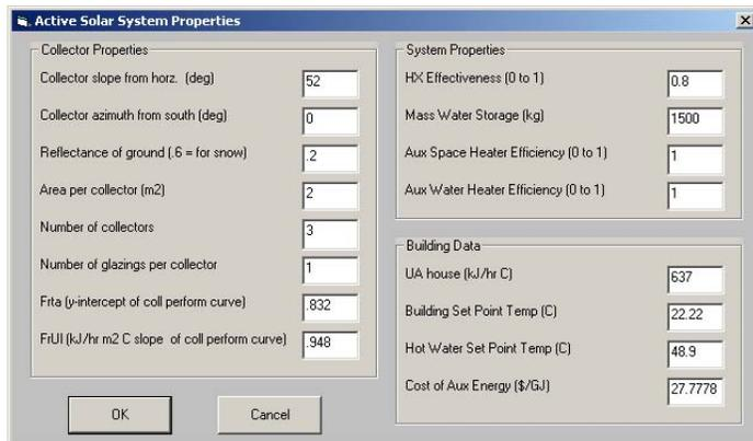
Figure 6. SolarSim input screen for modeling space and water heating.
