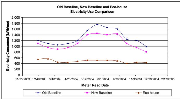
Figure 9. Comparison of electricity requirements for new baseline house and Eco-house.
