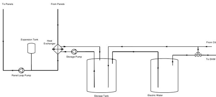
Figure 1: Solar Hot Water System
