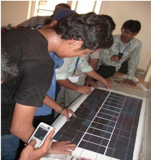
**Figure 3. PV cells laid on plain white printer paper in preparation for encapsulation**
