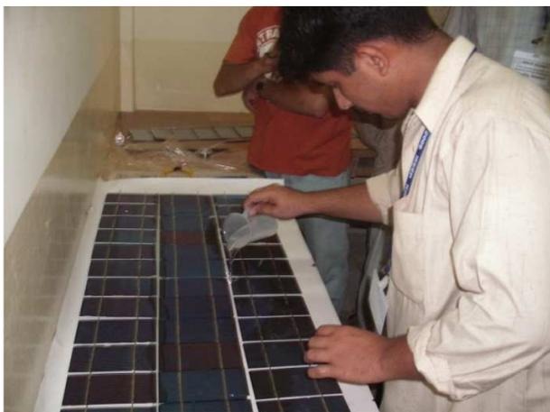
**Figure 4. Pouring the silicone to encapsulate the strings of cells**
