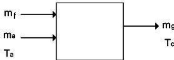
The energy balance reduces to the terms of inlet combustion air temperature,  $T_a$ , fuel lower heating value, LHV (about 21,500 Btu/lbm for natural gas), excess air, stoichiometric air
