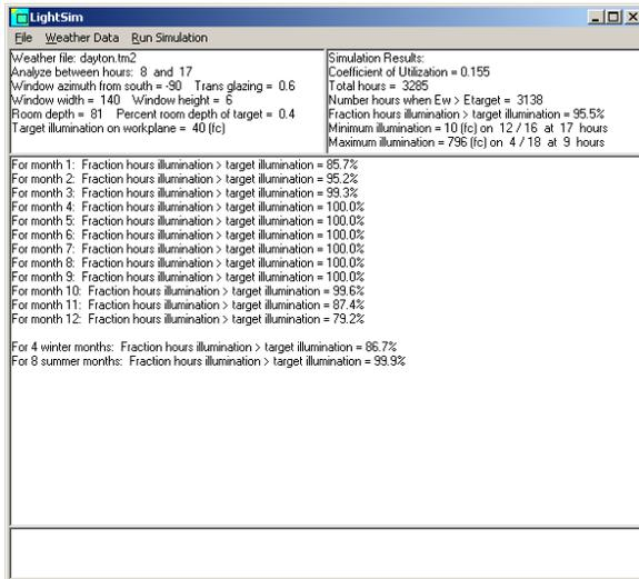
Figure 11. LightSim simulation results for foundry.
