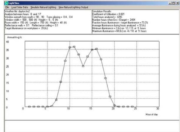
Figure 9. Simulated average lighting levels from natural light if the current windows were replaced with corrugated polycarbonate.
