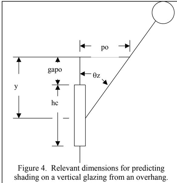
Figure 4. Relevant dimensions for predicting shading on a vertical glazing from an overhang.
