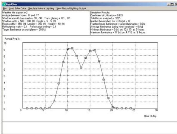
Figure 8. Simulated average hourly lighting levels from natural light, with current windows.
