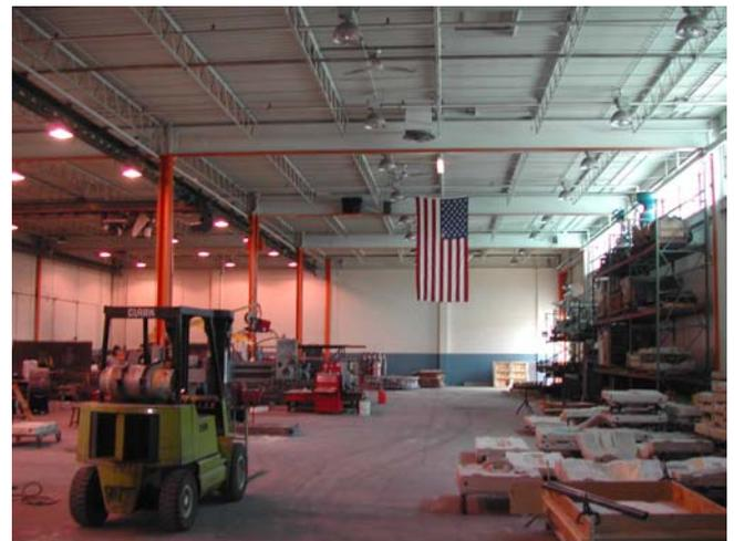
Figure 10. Foundry with east-facing windows that provide enough light to turn-off two of the five rows of lights.
