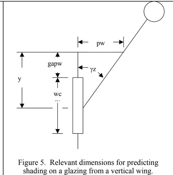
Figure 5. Relevant dimensions for predicting shading on a glazing from a vertical wing.
