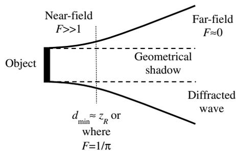
Fig. 1. Illustration of near- and far-field diffraction zones, along with minimum reconstruction distance  $d_{\min} \approx z_R$ , the Rayleigh range. The dashed lines show the geometrical shadow of the object, solid lines represent spreading due to diffraction.
