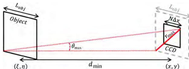
Fig. 2. Pseudo-3D illustration of the recording geometry given by Eq. (1). In this case, the maximum path length is the transverse projection,  $r_{\max}$ , on the CCD plane of the path from the lower left corner of the object to the upper right corner of the CCD array [1].
