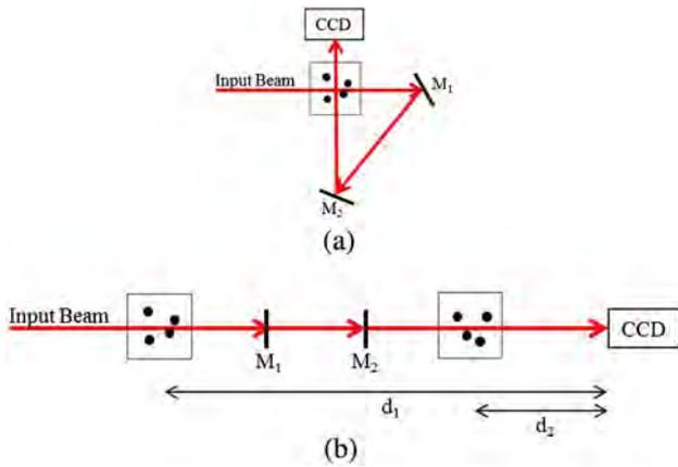
Fig. 7. (a) Schematic of single-shot multiple projection holographic tomography for recording and reconstructing the location of bubbles in water. (b) “Unfolded” version of the schematic in (a).
