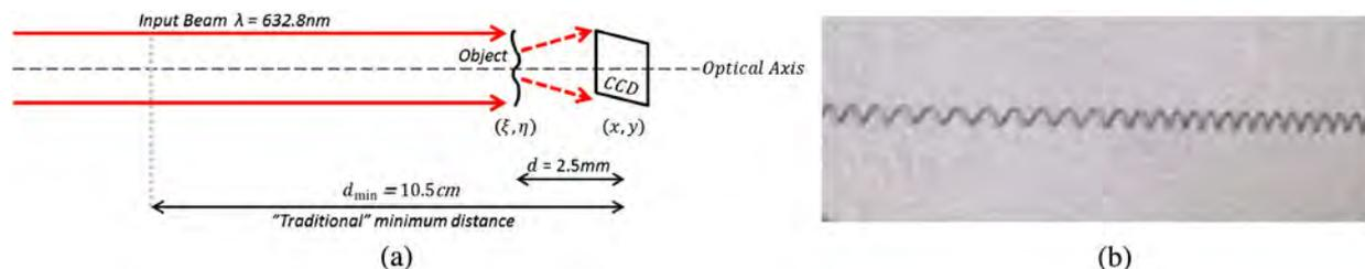
Fig. 3. (a) Near-field, in-line (Gabor) recording geometry, and (b) photograph of the tungsten filament object.
