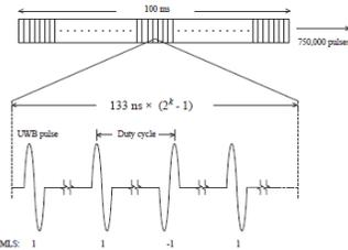
Fig. 2. BPSK-modulated pulse train with an MLS.
