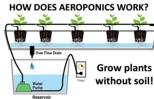
Figure 2: Diagram of aeroponics system
