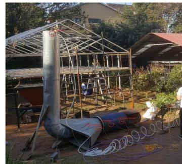
Figure 2. Burn Trial and Thermocouple Setup
