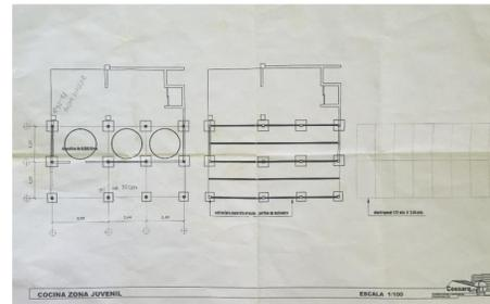
Figure 2: Design for kitchen expansion with water tanks
