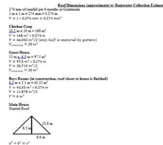
Figure 4: Rainwater collection system dimensions and collection calculations
