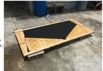
Figure 6: Unassembled Solar Dryer
