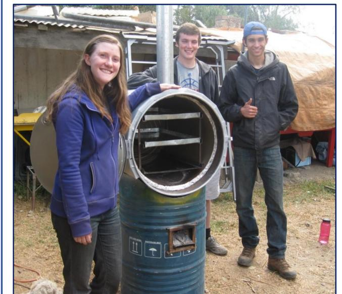
Figure 3. Completed ETHOS Rocket Oven
