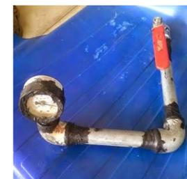
Figure 3: Knifing Paste and Natural Fiber Test
