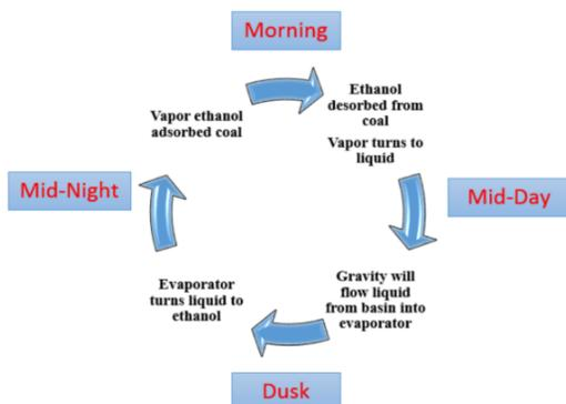
Figure 1: Daily Adsorption Cycle
