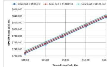
Net Present Value of lifecycle system costs at 6% discount rate for Hybrid GCHP
