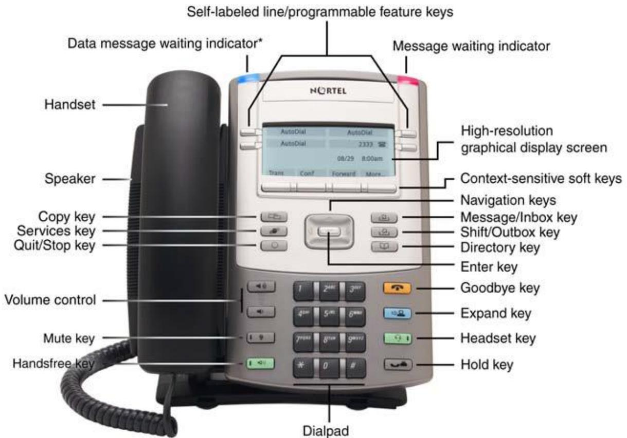
**Context-sensitive soft keys** are located below the display area. The LCD label above each key changes based on the active feature. The only key that can't be changed is the Prime DN key (the main line). When a triangle appears before a soft key label, the feature is active.
