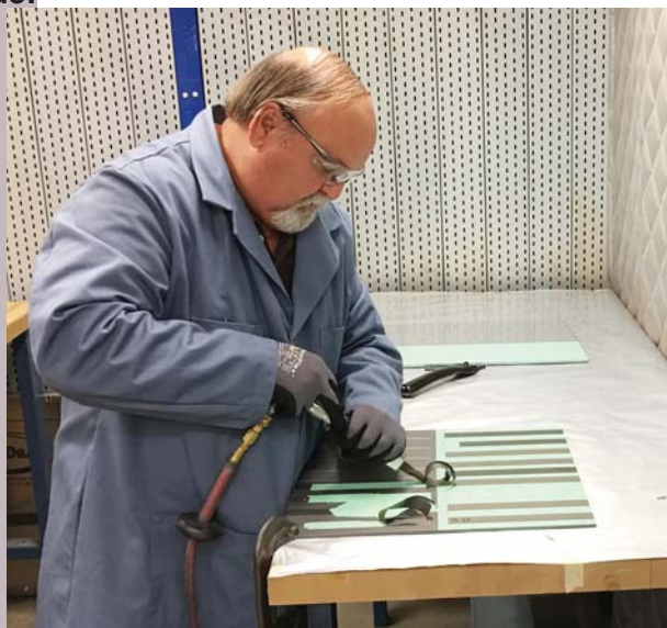
Paul Childers uses a specialized tool he developed to remove elastomer tape and coating without damaging the underlying composite substrate.
