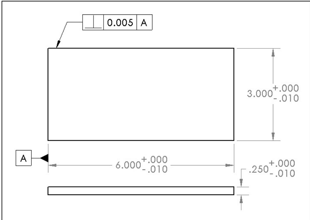
Figure 7: Rectangular Specimen – Configuration 2
