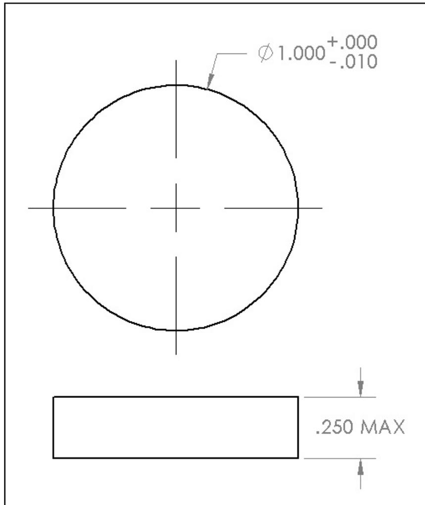
*Figure 5: Round Specimen – Configuration 1*
