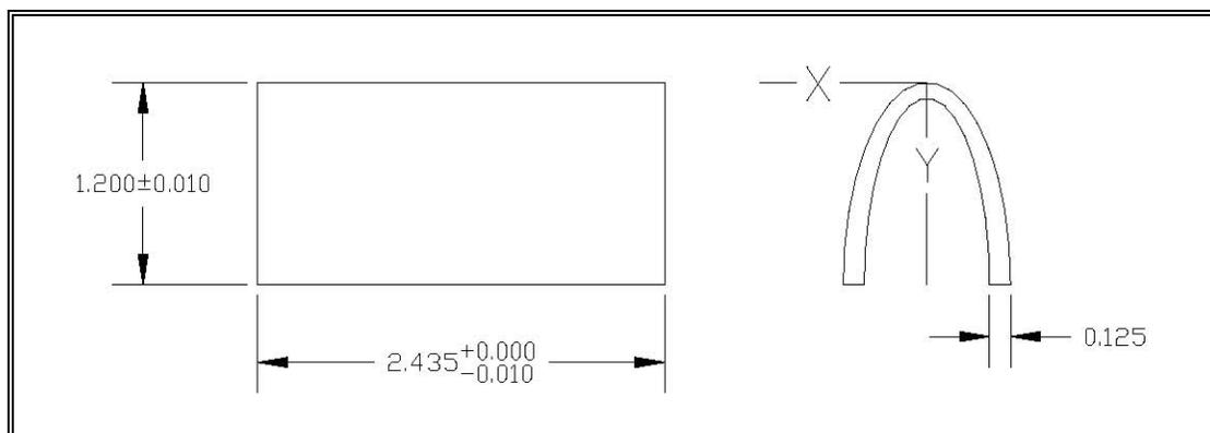
Figure 9: Metallic Leading Edge Airfoil Specimens – Configuration 1
