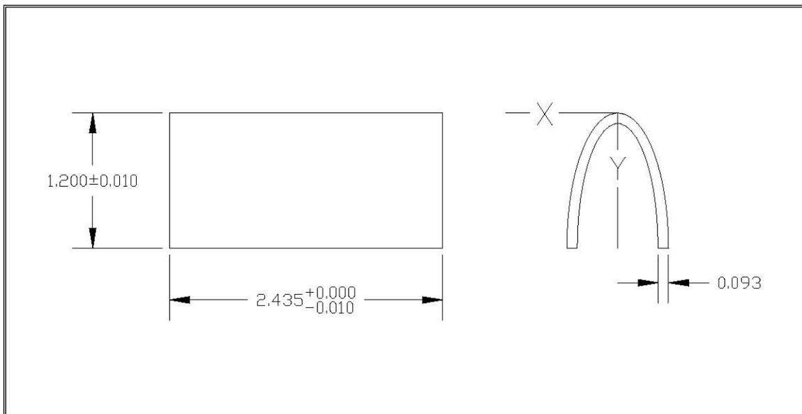
Figure 8: Composite Leading Edge Airfoil Specimens – Configuration 1
